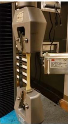
Fig. A.24: (Left) Mechanical testing of membrane specimens (middle). (Right) An example output of the results from the mechanical testing. Even though this schematic shows only monotonic, also creep and fatigue tests have been carried out.
