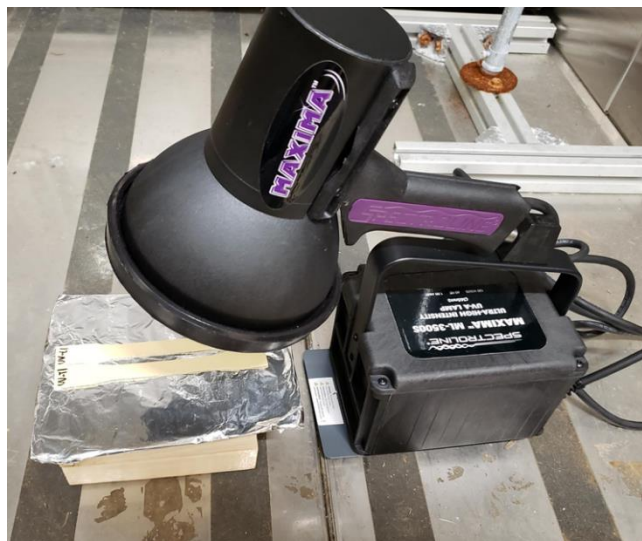
Fig. A.25: Accelerated UV-degradation test set up using a ML-3500S UV-A lamp. One specimen of each orientation is placed 4.75” from the UV source, resulting in an irradiance of approximately 5014 W/m 2 . Light has been turned on for clarity in this picture, but actual setup is in the dark.
